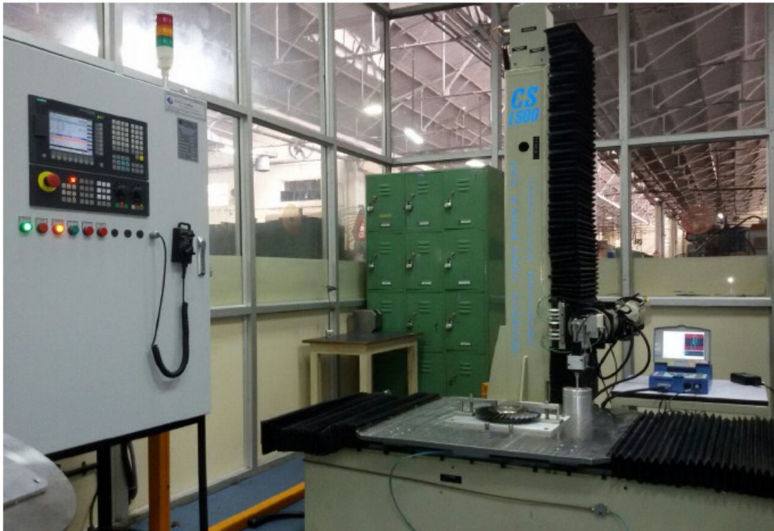
Fig4. Automated Eddy Current Inspection Set up with CNC based Up and Down System
