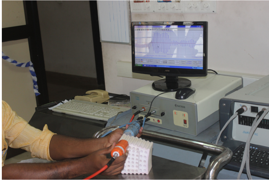
Fig 1: Evaluation of cored bricks for storage heaters.
